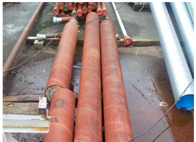
Picture of 7" tubings cemented inside 9 5/8" casings.
