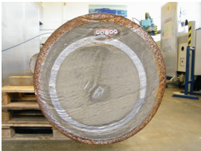
Picture of 7" tubing cemented inside 9 5/8" casing. Good cement placement is obtained when tubing is left in hole.
